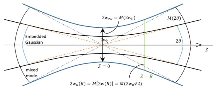
Figure 2 – Embedded Gaussian concept
